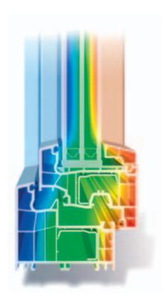
Three-dimensional illustration of distribution of heat through a window cross-section.
